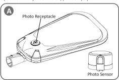
If the fixture with PHOTO CONTROL function, the Photo Receptacle will be installed on the cover of fixture. See (A). Fit the pins of Photo Sensor to Photo Receptacle, firmly insert and rotate Photo Sensor to proper position.
